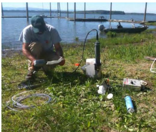
USGS technician taking water quality readings for dissolved oxygen, temperature, pH, and conductivity from a shallow groundwater well installed at the Vancouver Lake Sailing Club.
