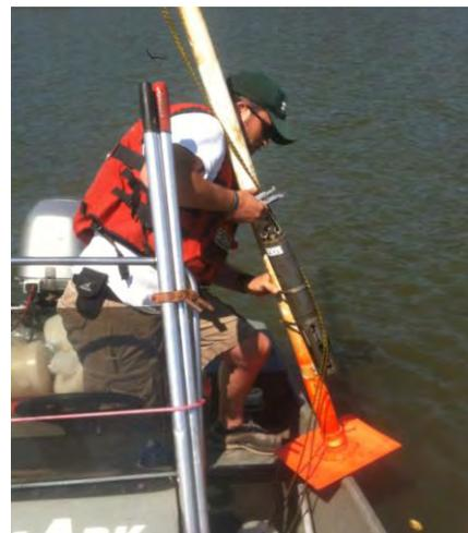
USGS technician retrieving turbidity sensor to download data and clean for redeployment.
